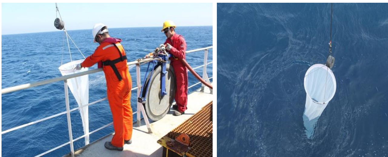
Figure 5-5 Representative Photos of Plankton Sampling Equipment and Procedures from the Primary Marine Baseline Surveys
