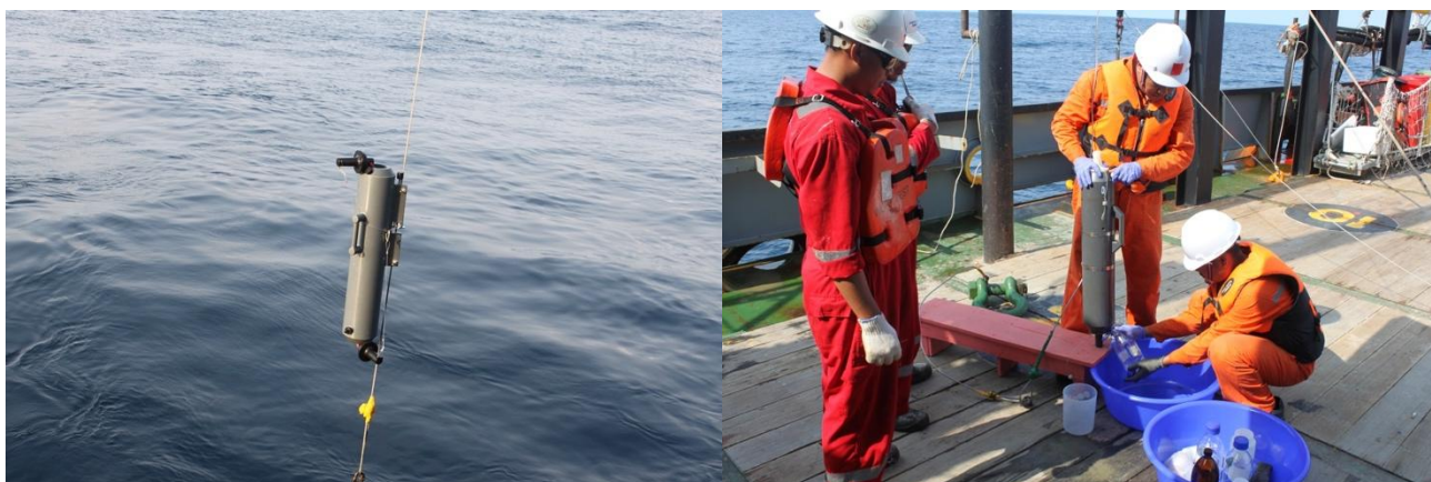
Figure 5-3 Representative Photos of Seawater sampling Equipment and Procedures from the Primary Marine Baseline Surveys
