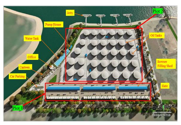
Figure 4.3. Layout Plan of the Proposed Project
