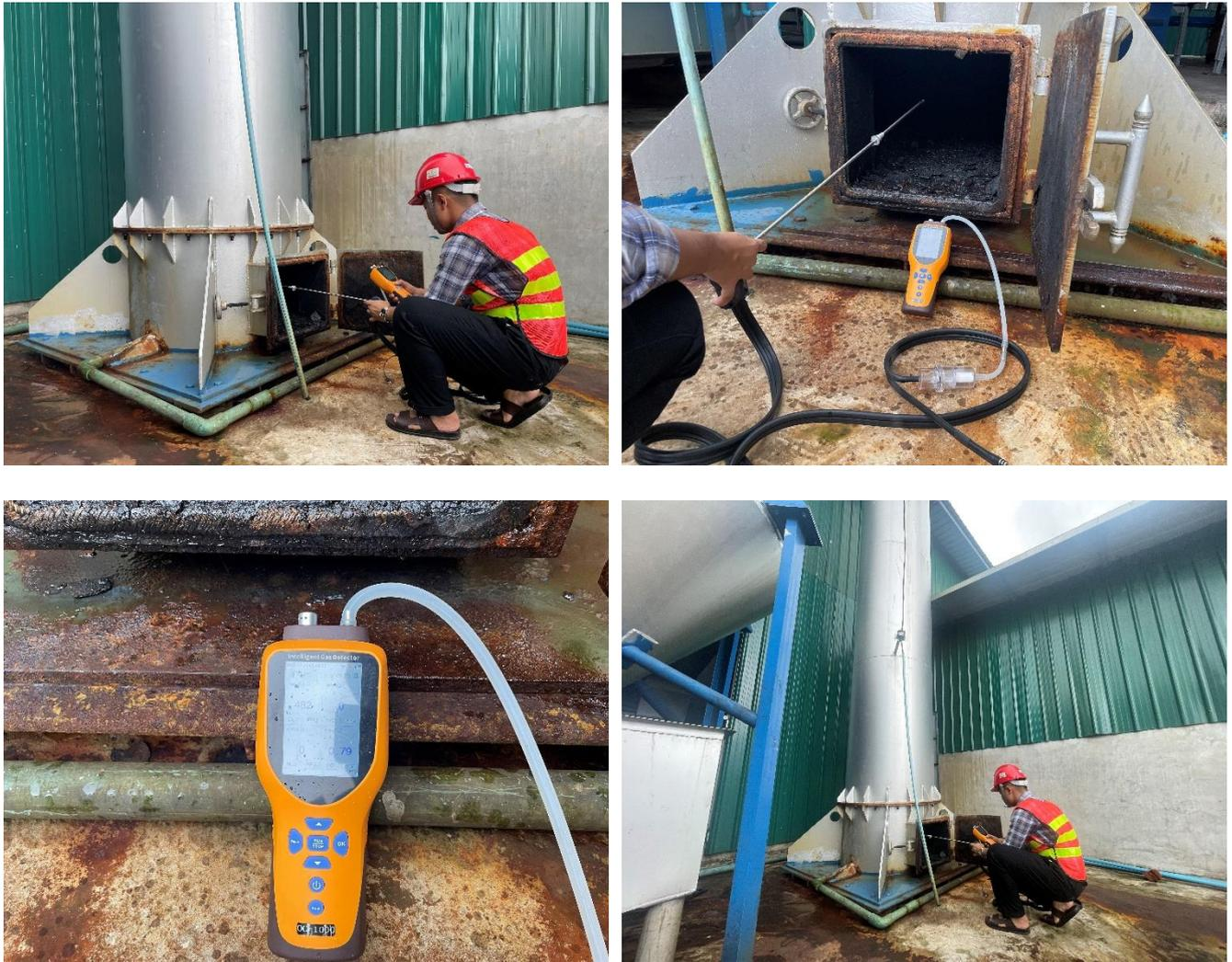
**Figure 4-15 Boiler Stack Emission Measurement Photos**
