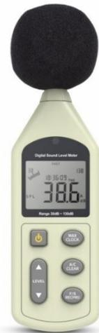
Figure 4-11 Digital Sound Level Meter (BENTECH, GM – 1356)
