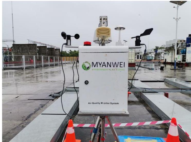
Figure 4-9 Air Quality Monitoring System (Oceanus AQM-09)
