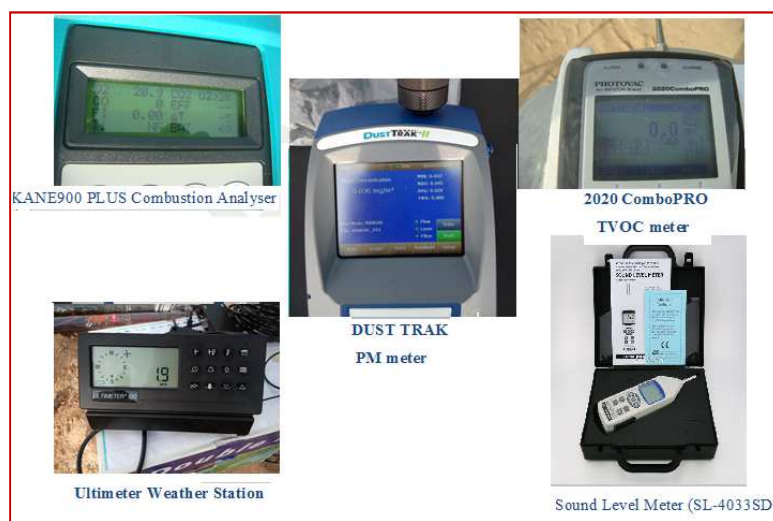
Figure 3.6 Equipment used for surveying the Air Quality and Noise Level Baseline Data
