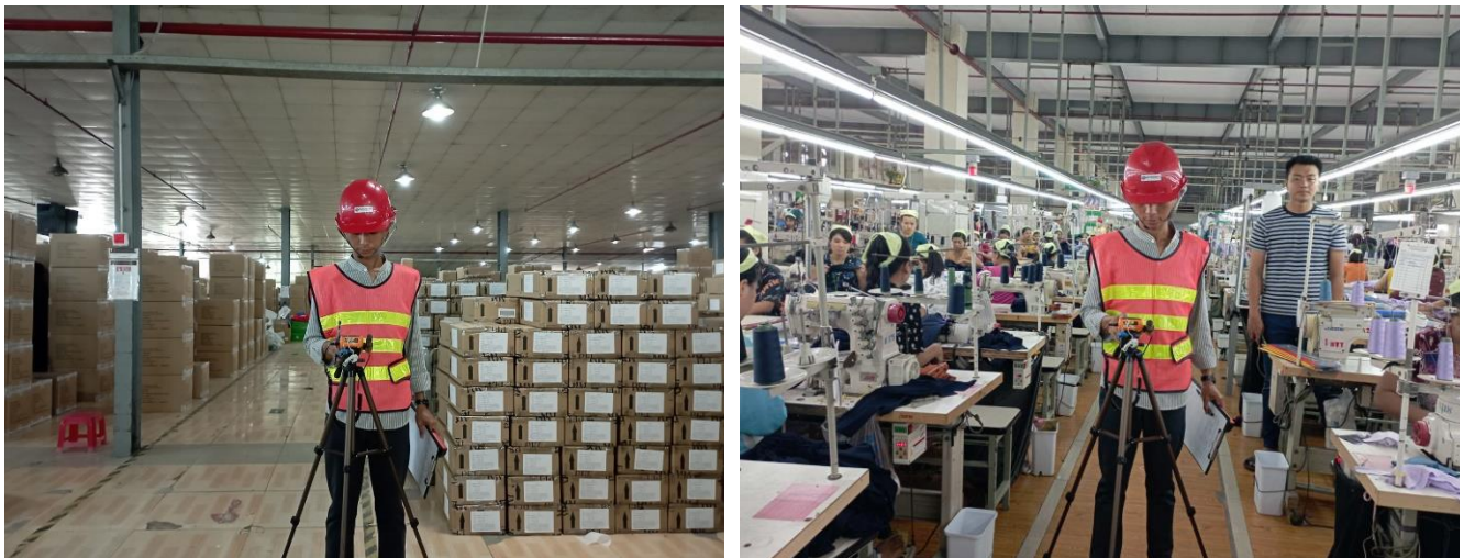
Figure 5-11 Temperature and Relative Humidity Measurement Photo
