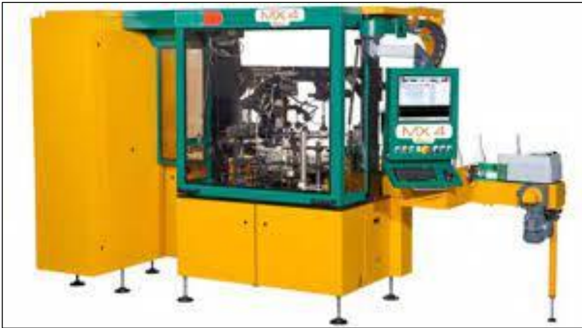
Figure 3-26 M1 Inspection Machine for Side Wall Inspection
