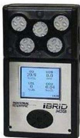
Plate 5.23 Portable multigas meter used to monitor sulfur dioxide (SO 2 ) and nitrogen dioxide (NO 2 )
