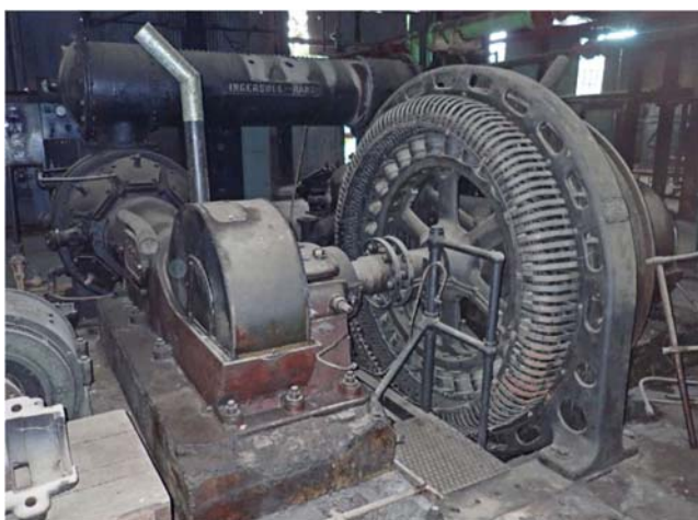
Plate 5.68 Ingersoll-Rand air compressor and synchronous motor in the compressor house
