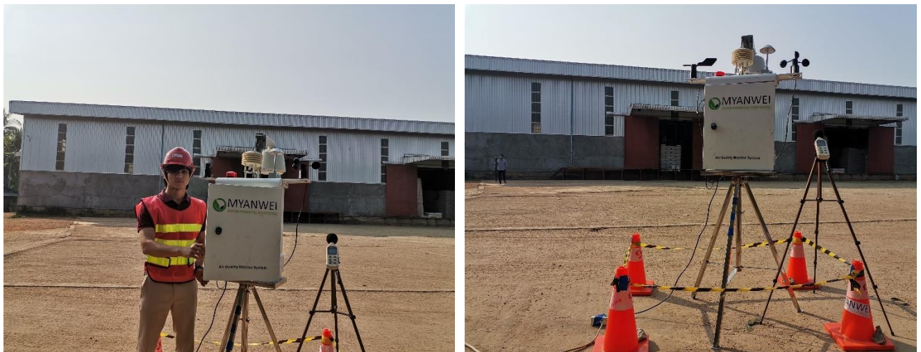
Figure 5-2 Outdoor Air Quality Monitoring at Project Site
