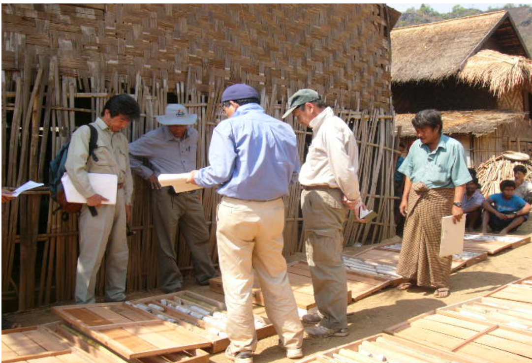
Photo(6) Drill core examination ( Neo Energy Development Co., Ltd & Nippon Koei consultant team )
