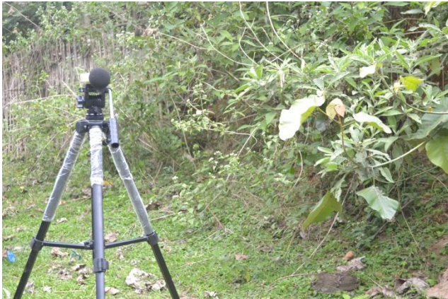
Noise Level Measuring by Digital Sound Meter
