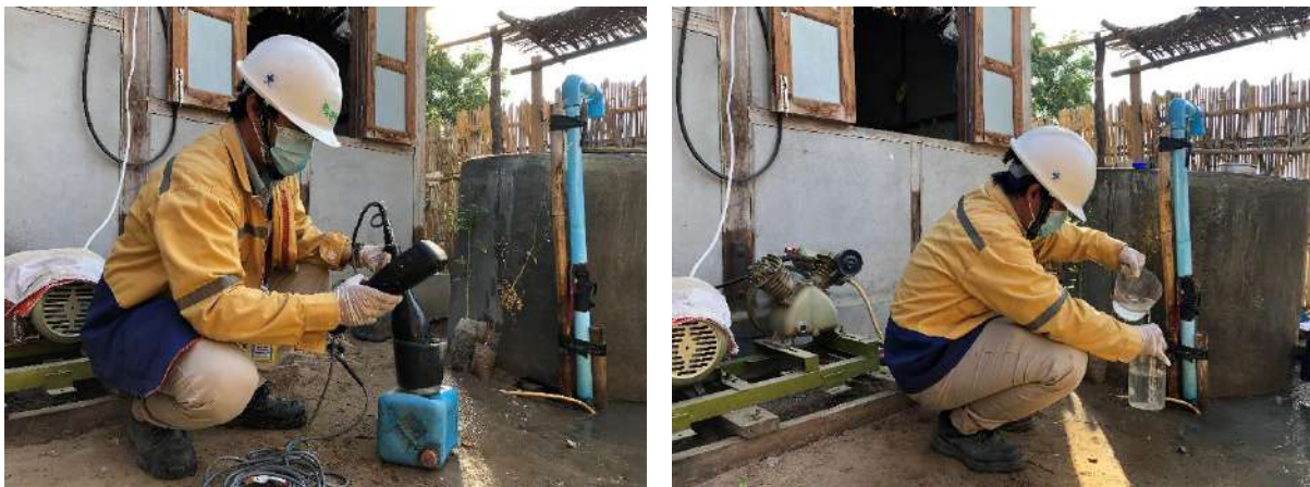
Figure 6. 11 On-site Water Quality Measurement and Water Sampling
