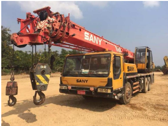
Mobile Crane (25 T)
