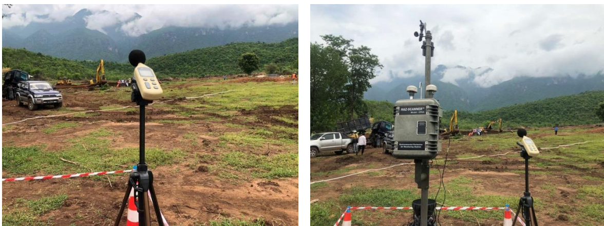
Figure 6. 12 Noise Level Monitoring at the Proposed Project Site
