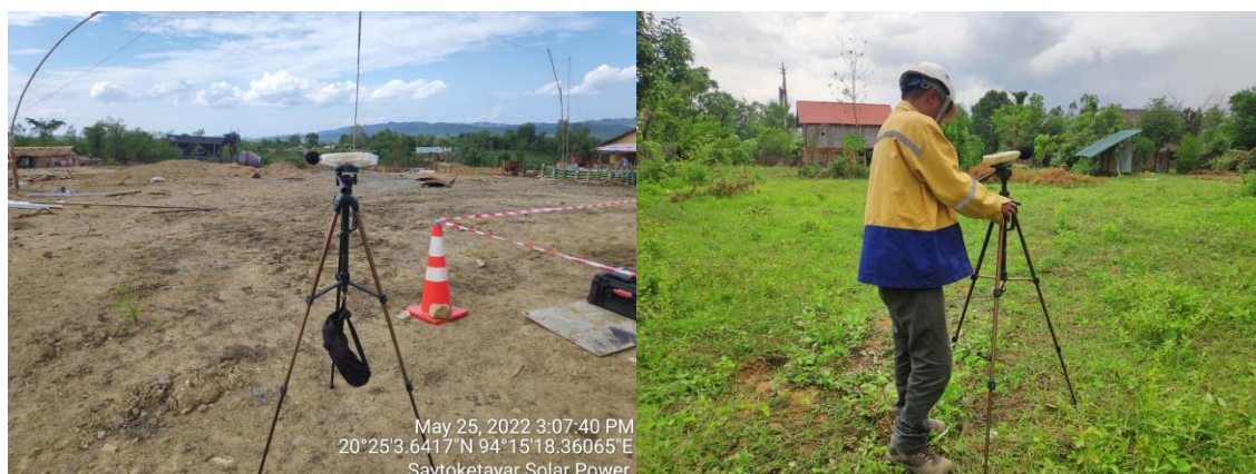
Figure 6. 9 Noise Level Monitoring at Source and Receptor of the Proposed Project
