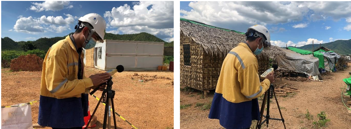
Figure 6. 12 Noise Level Monitoring at Point 1 and 2 of the Proposed Project
