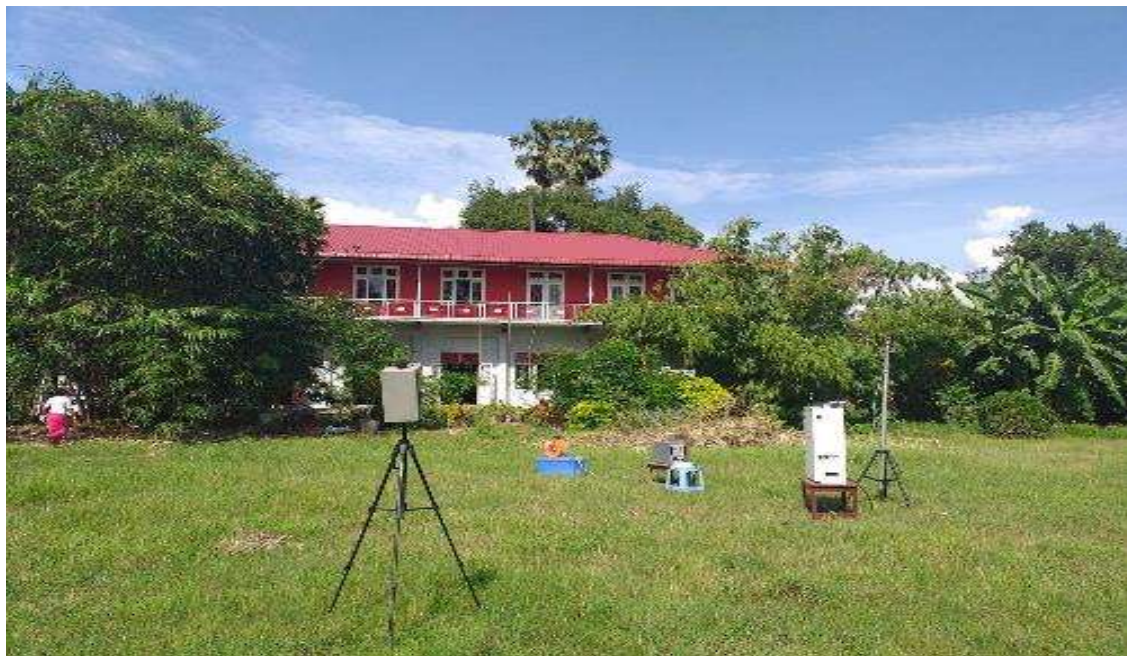
Figure 5.9: Noise monitoring station at the Inn Jal village
