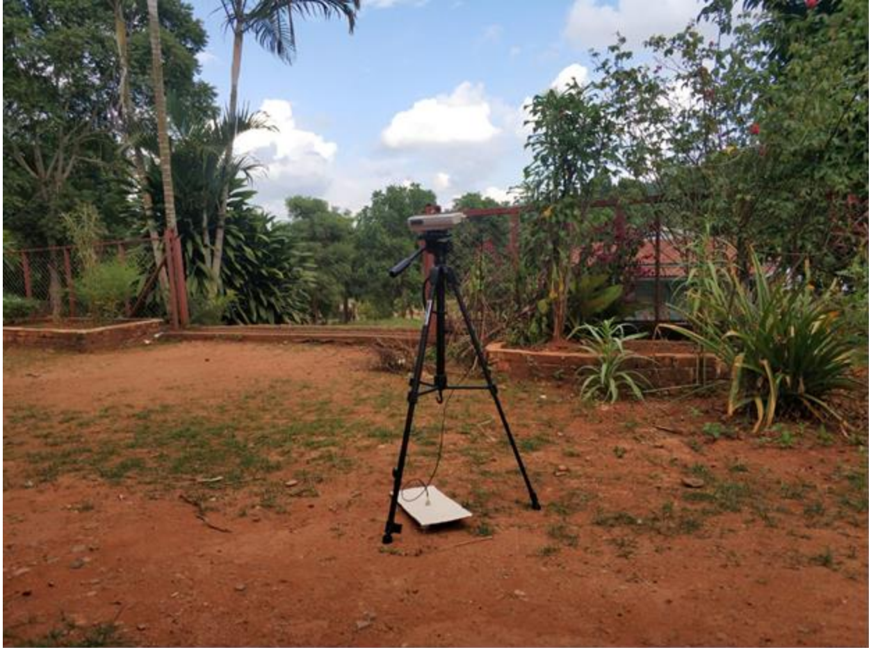
Figure 4: Natura vibration level monitoring
