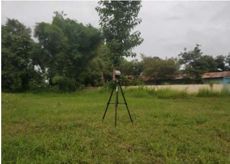
Figure 5.11: Vibration monitoring station at the Inn Jal village
