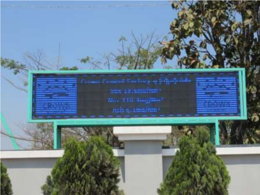
Figure – 34: LCD signboard installed near the gate showing results of continuous monitoring
