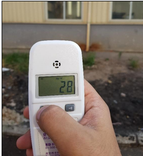
Figure 6-1: Air Quality Monitoring Near the Boiler
