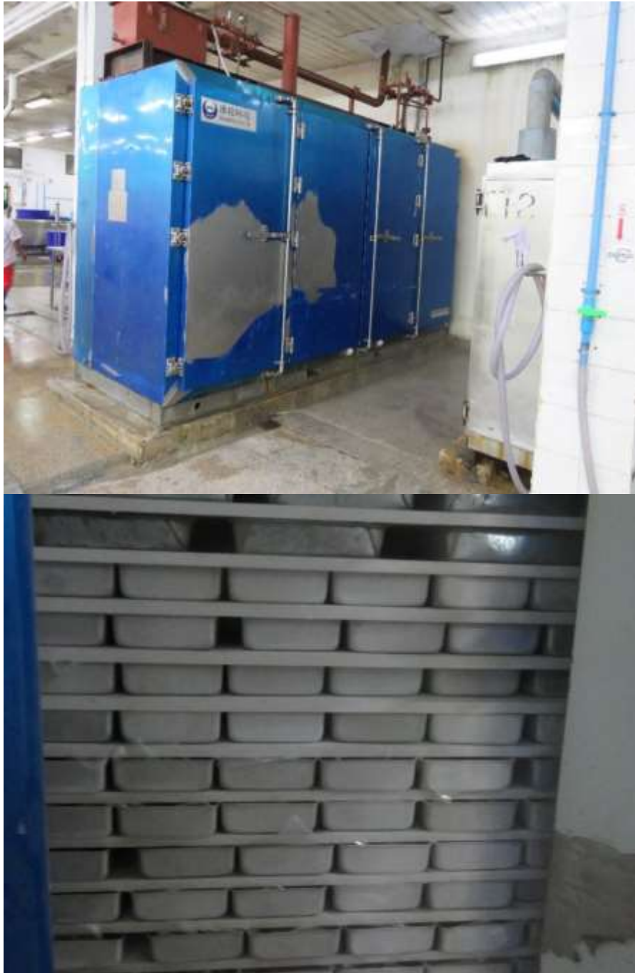
Figure 4. 33 Freezing at a temperature below - 35°C
