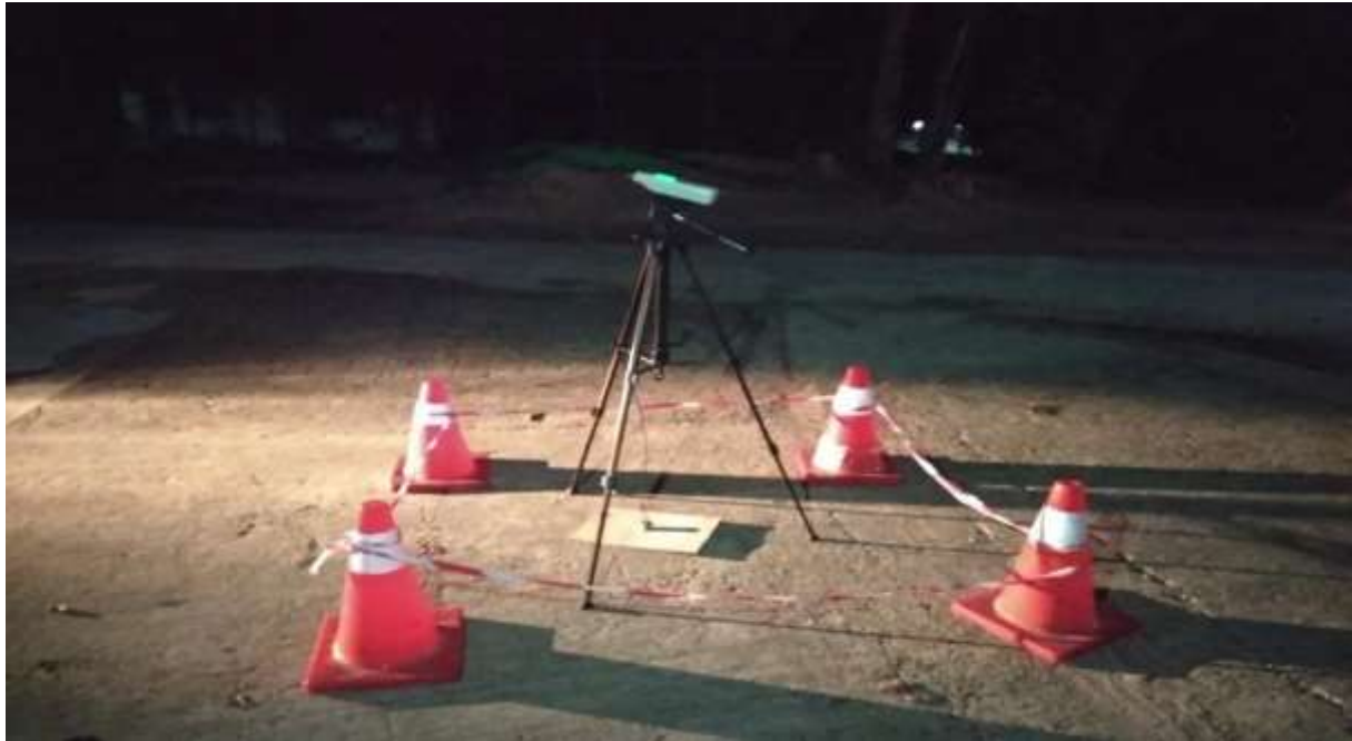
Figure 5. 27 Vibration monitoring station at Nan Taw monastery (Night time)
