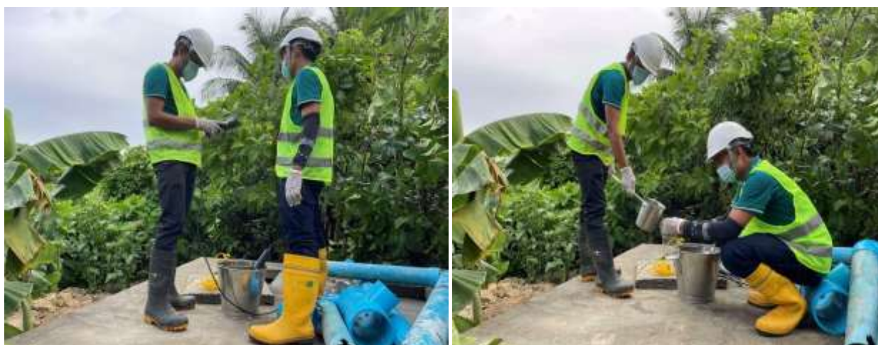
Figure 5. 39 Effluent water sampling
