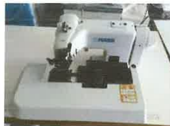
COMPUTER CONTROLLED, HIGH SPEED, LOCKSTITCH, BUTTON HOLDING MACHINE (COMPLETE SET)
