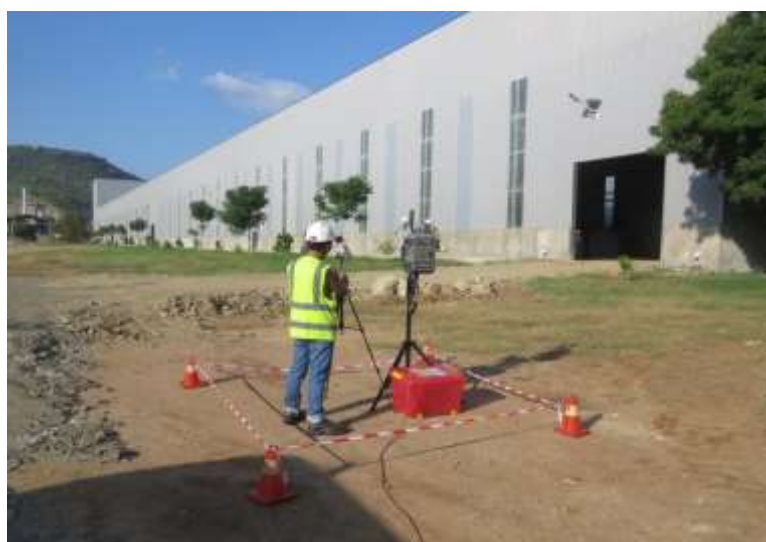
Figure – 74: Measuring air quality at proposed site
