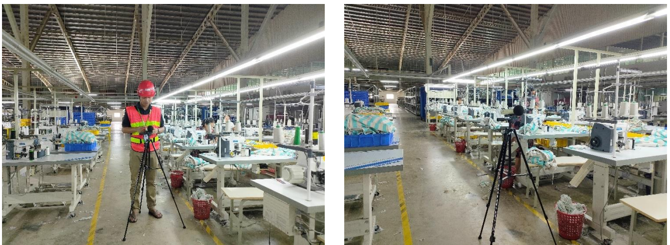
Figure 4-8 Sound level measurement photo
