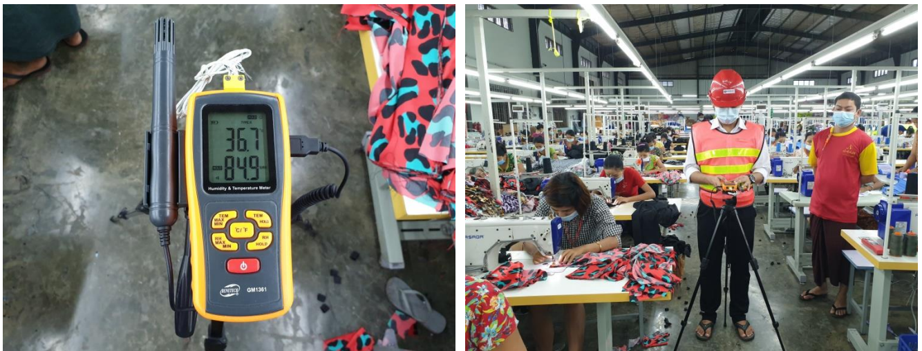
Figure 4-4 Temperature and Humidity Measure Photo
