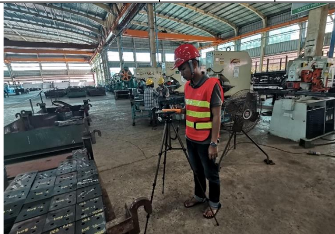
Figure 4-6 Temperature and Humidity Measurement in Operation Area
