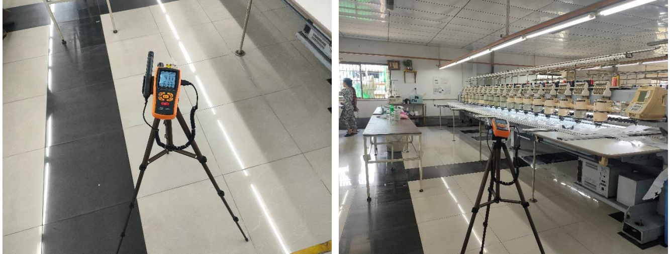
Figure 5-5 Temperature and Relative Humidity Measurement Photo
