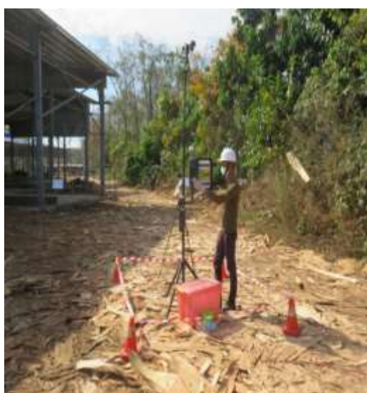
Figure – 21: Measuring air quality at project site during day time
