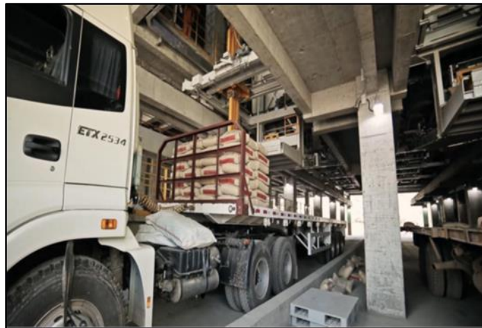
Figure 4.14 Bags Car Loading (Auto Machine)
