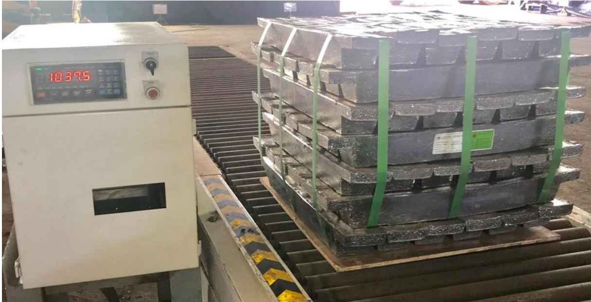
Figure 3.6-8: Bundle Weighting System with Printer
