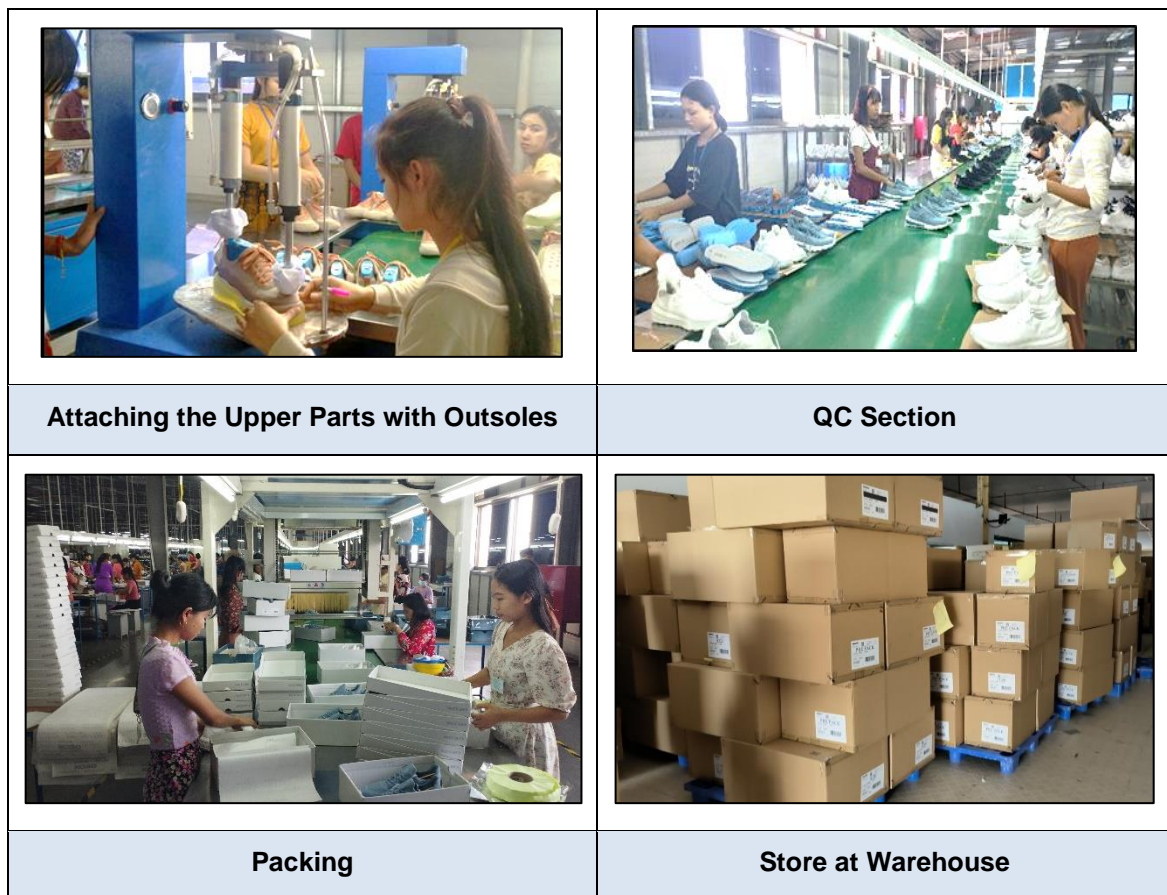
Figure 3-14 Lasting and Packing Processes
