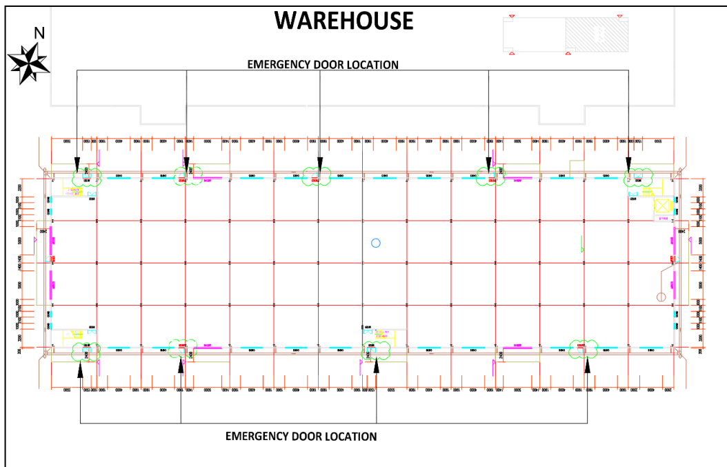
Figure 3-25 Emergency Door Plan for Warehouse Building
