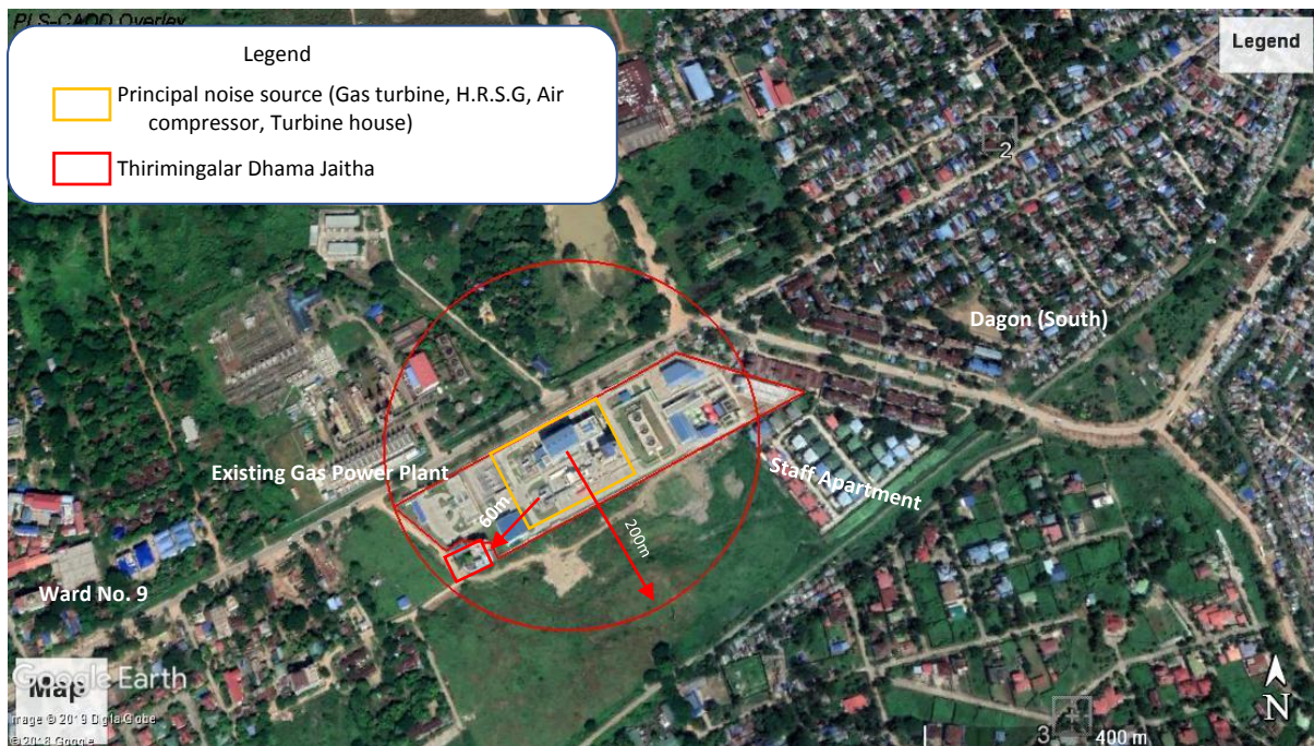
Figure 7.3-5 Principal Noise Sources During Operation Phase Compare with The Surrounding Noise Receptors
