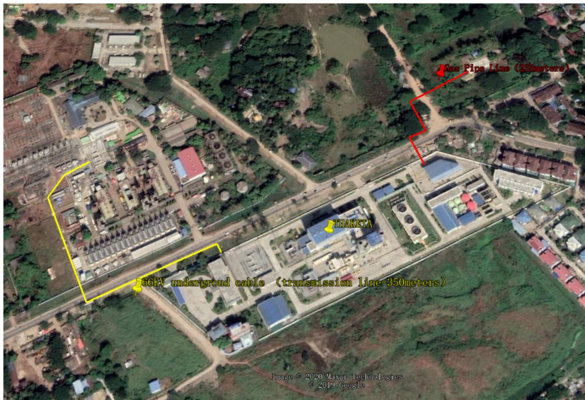
Figure 3.4-1: 66kV Transmission Line and Gas Intake Pipeline
