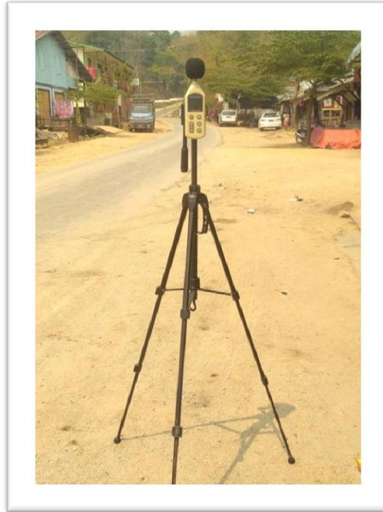
**Figure 5. 6: Noise quality Measurement at Sin Maung village for 24 hrs (continuously)**
