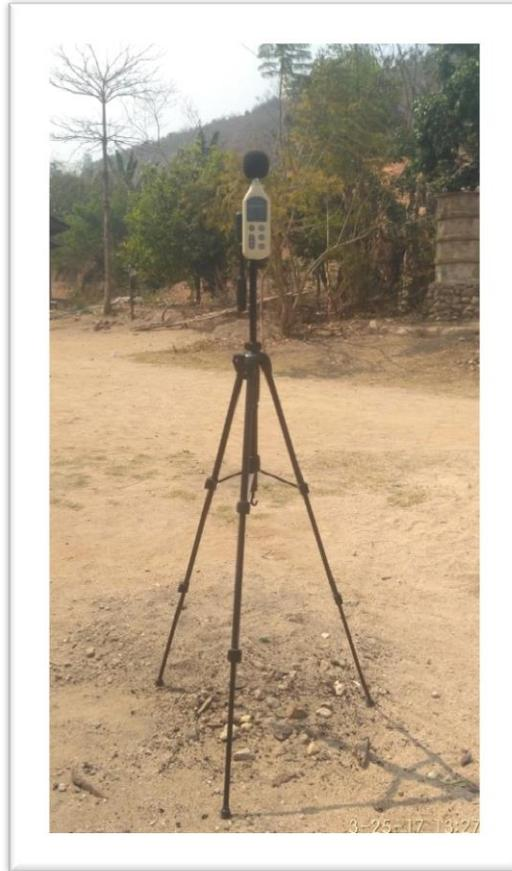
**Figure 5. 4: Noise quality Measurement at Pan Kyuu village for 24 hrs (continuously)**
