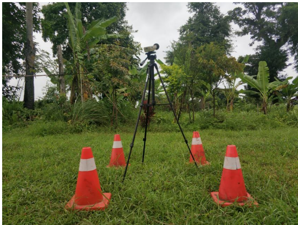
Figure 3.4 Noise monitoring station at the Cha Ya Gone village
