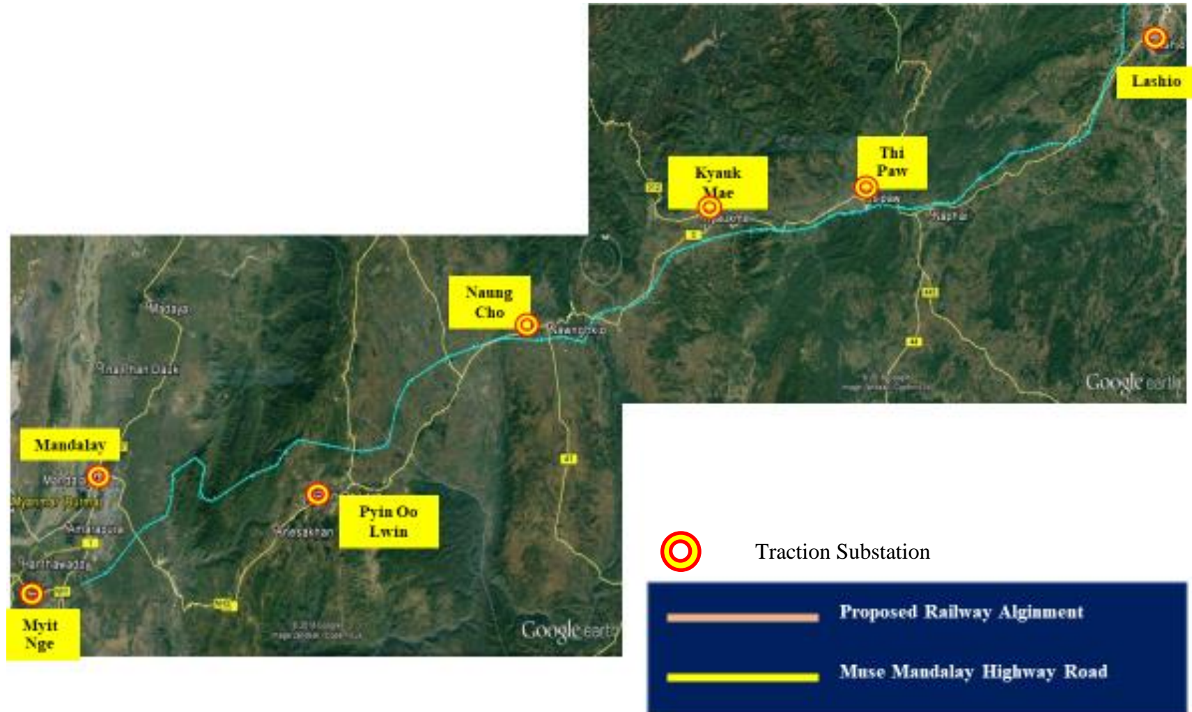
Figure 3.1 Muse-Mandalay Railway Alignment and Power Transmission Line in Google Earth (Mandalay to Lashio)
