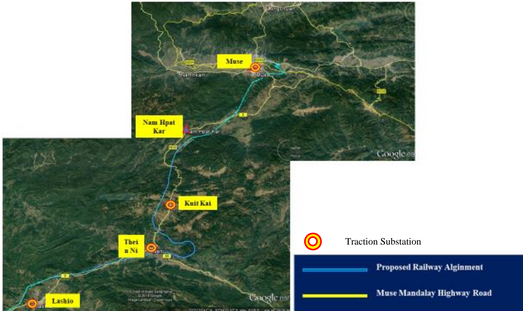
Figure 3.2 Muse-Mandalay Railway Alignment and Power Transmission Line in Google Map (Lashio to Muse)
