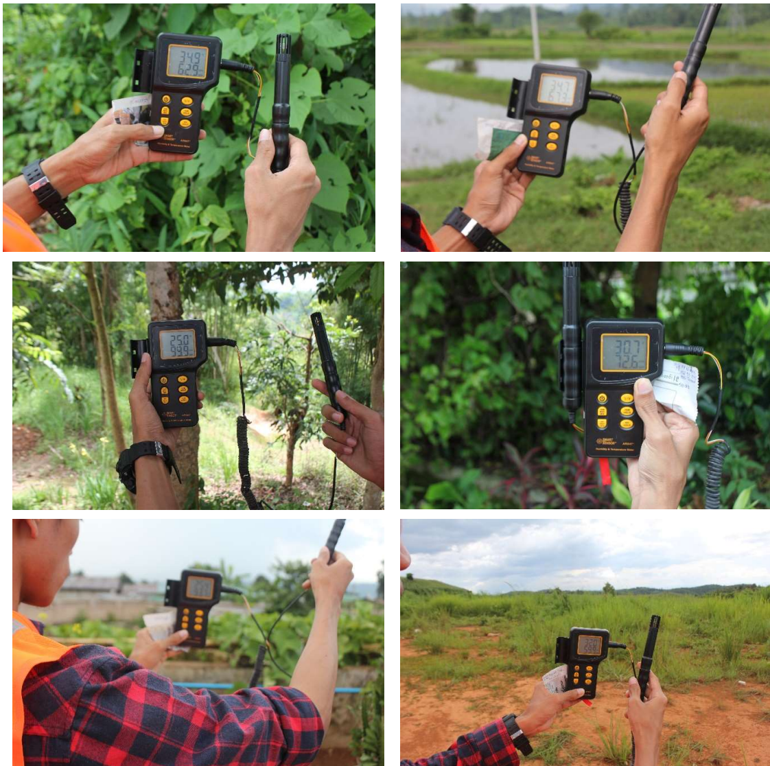
Figure 5.17 -Recorded Photos about measuring temperature and air humidity
