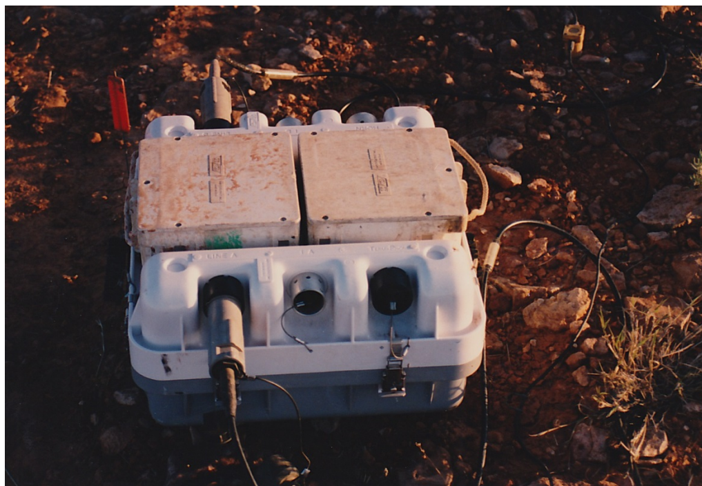
Figure 4.14 A line "box" that collected the signal from 6 geophone strings before transmitting along the fibre optic cable to the recording instrument
