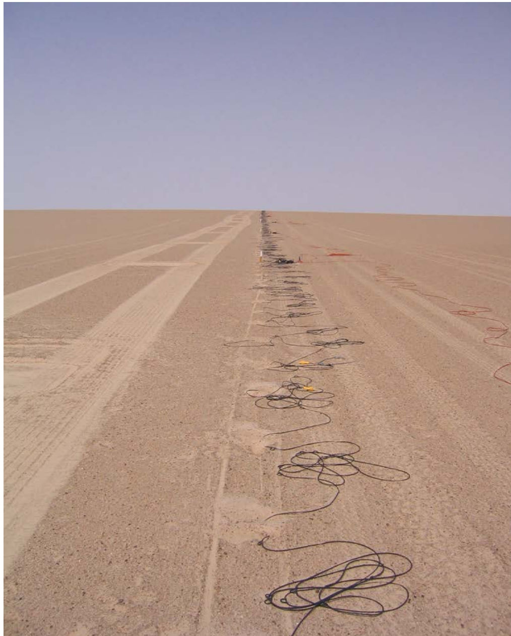
Figure 4.11 Example of a 2D seismic line in a desert environment immediately after recording. Note the vibrator pad marks and wheel tracks on the left and the geophone cables in the centre with the fibre optic cable to the recording instrument on the right.
