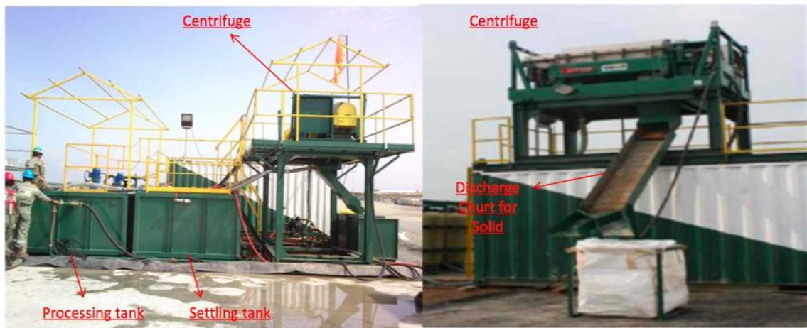
Figure 4-27: Centrifuge Process and Steps
