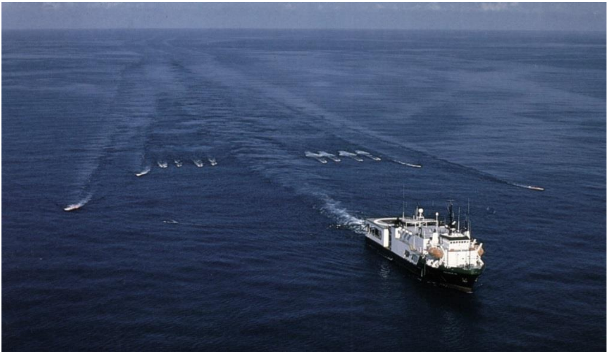
Figure 4-2: Typical 3D Survey Spread
