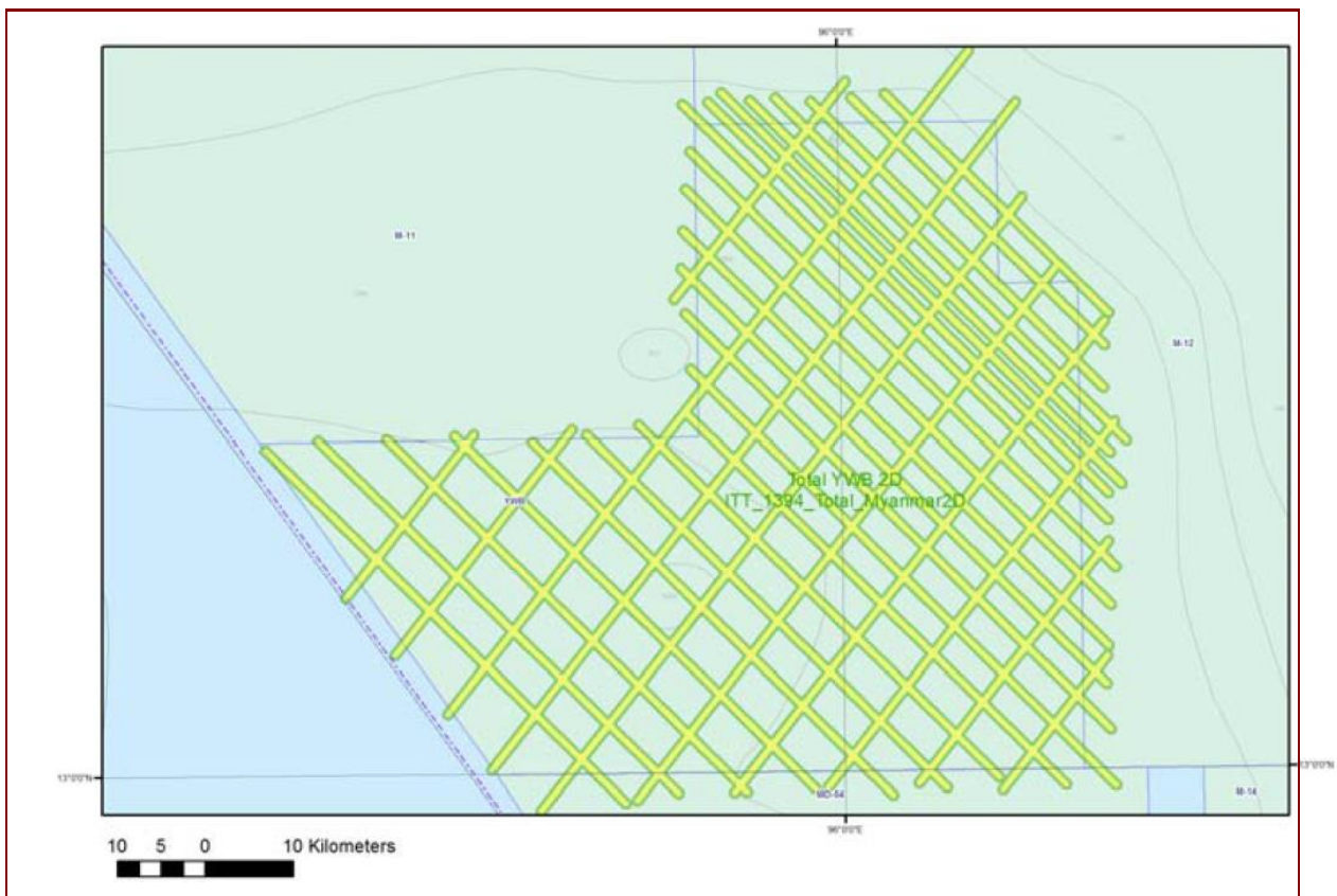
Figure 2-4 Racetrack shooting pattern for the 2D seismic survey (Alternative)
