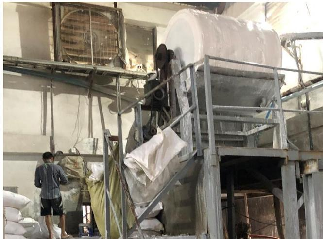
**Figure 3-5 Photo of Mixing Machine**
