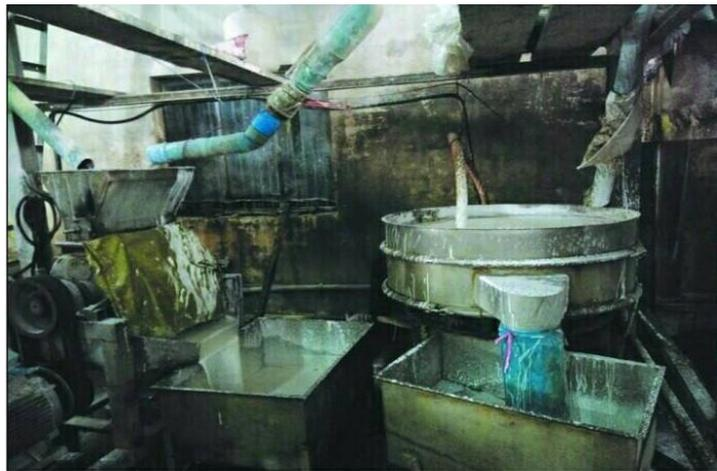
**Figure 3-3 Photo of Rice Grinding Machine**
