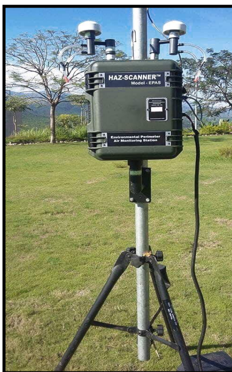
Figure 4.3 Air Quality Monitoring Device
