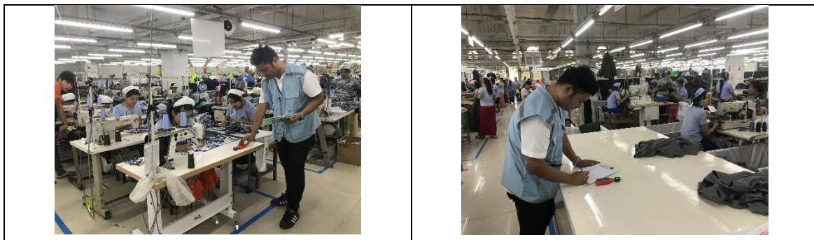
Figure 4-16 Light measurement in working lines of building A
