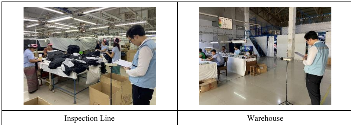
Figure 4-11 Noise level measurement in the garment factory
