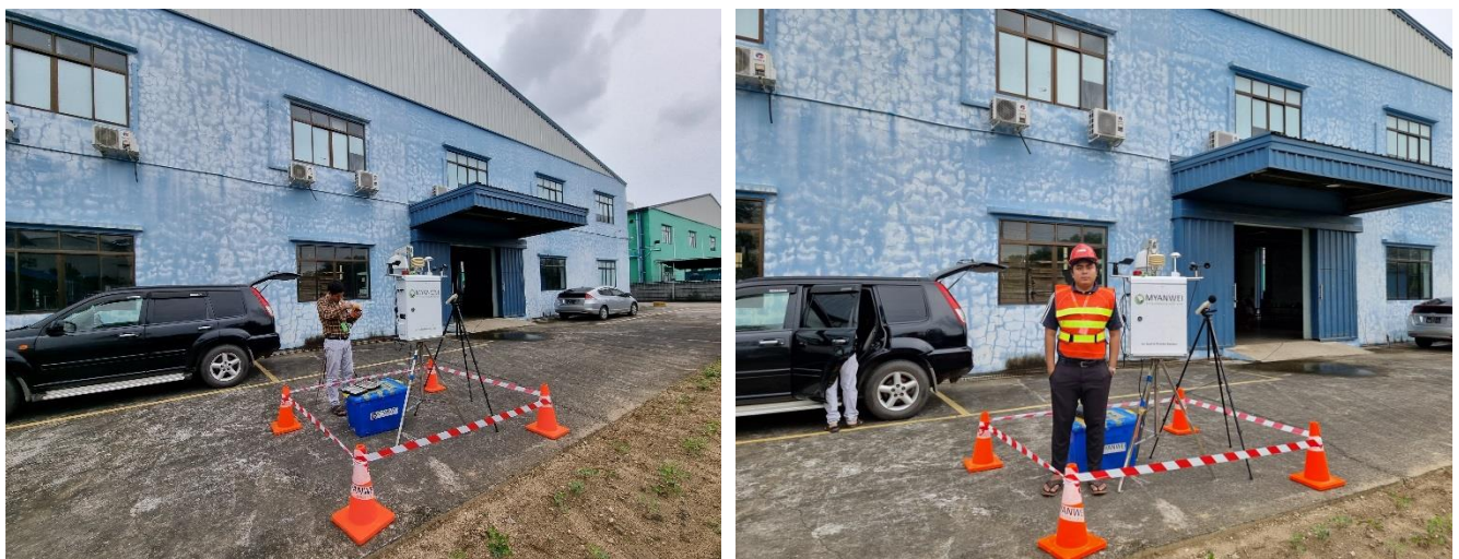
Figure 4-7 Sound level measurement photo
