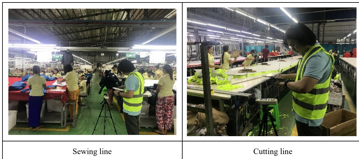
Figure 4-15 Noise Level Measurement in the Garment Factory
