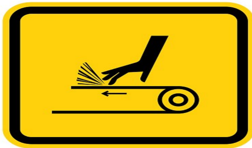
Figure 5-12 Stick the warning sign near the hand abreaction belt drive
