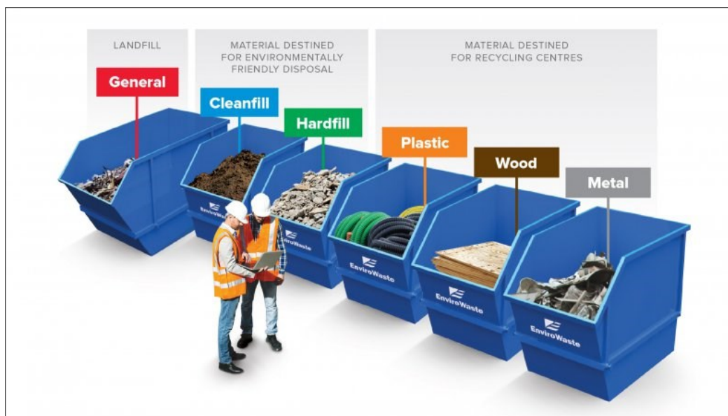
Figure 5-4 Example of Construction solid wastes separated at the construction site
