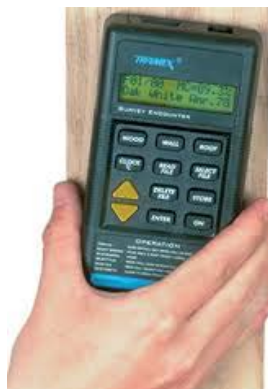
Figure 2.3 Tramex moisture meter
