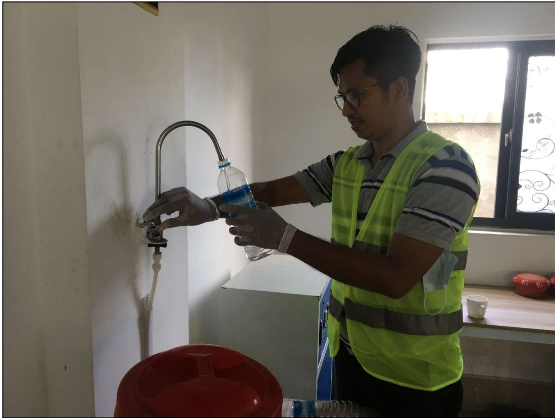
Figure 1-8 Water Sample Collected from Drinking Water Pipe
