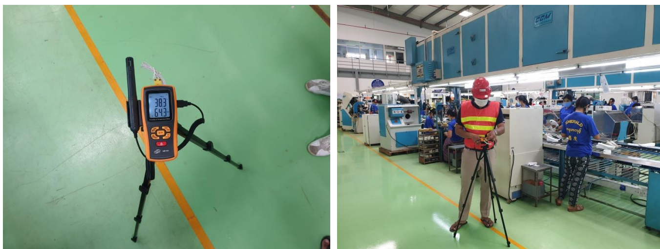
Figure 6-5 Temperature and Humidity Measurement in Operation Area of the Factory
