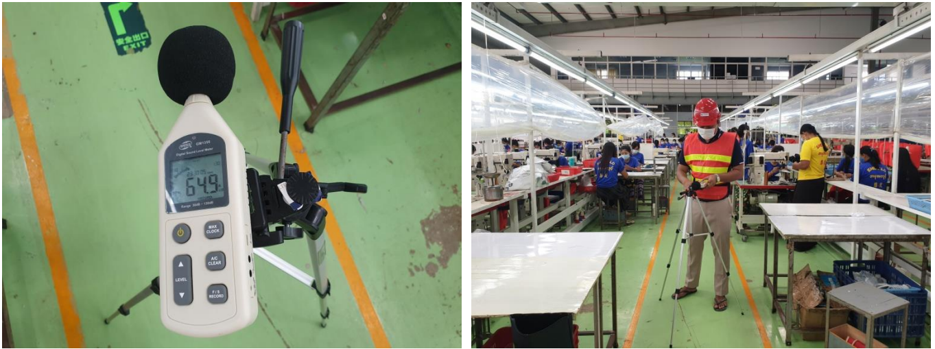
Figure 6-2 Noise Level Measurement Photo
