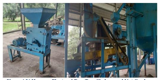
Figure 4.24 Hammer Plant and Two Tray Shakers and Nut Crackers
