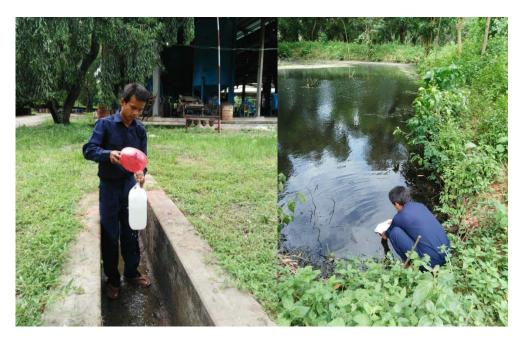
Figure 5.13 Drainage Water and Final Treated Water Samples Collection during Rainy Season
