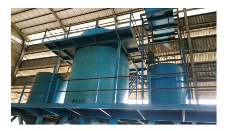
Figure 4.48 Photo of Oil Separation Tank
