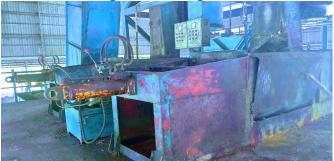
Figure 4.37 Double Screw Press
