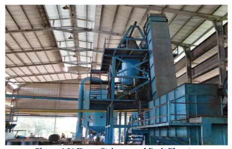
Figure 4.21 Drum Stripper and Fruit Elevator
