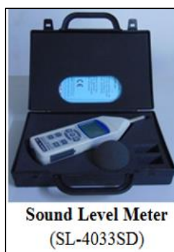
Figure 4-11 Equipment used for Surveying the Noise Level
