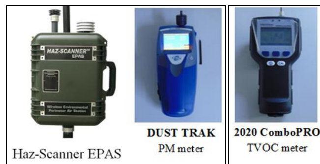
Figure 4-1 Equipment used for Surveying the Air Quality
