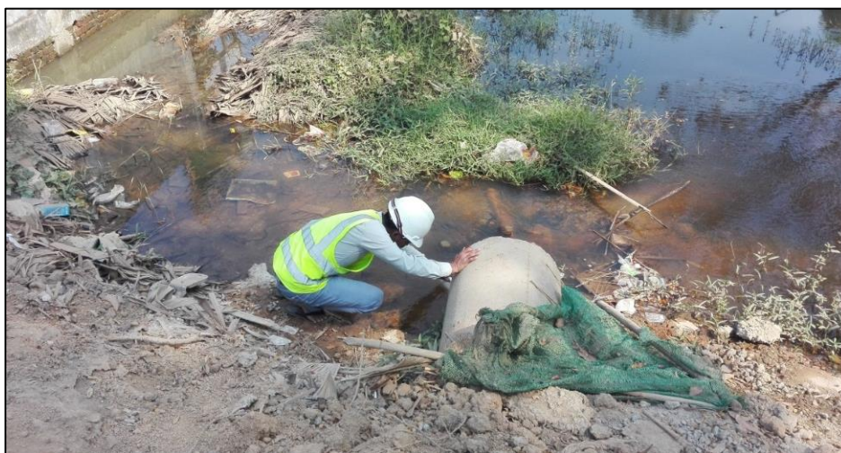
Figure 4-8 Photo of Taking Wastewater Sample from Municipal Drain in front of the Factory
