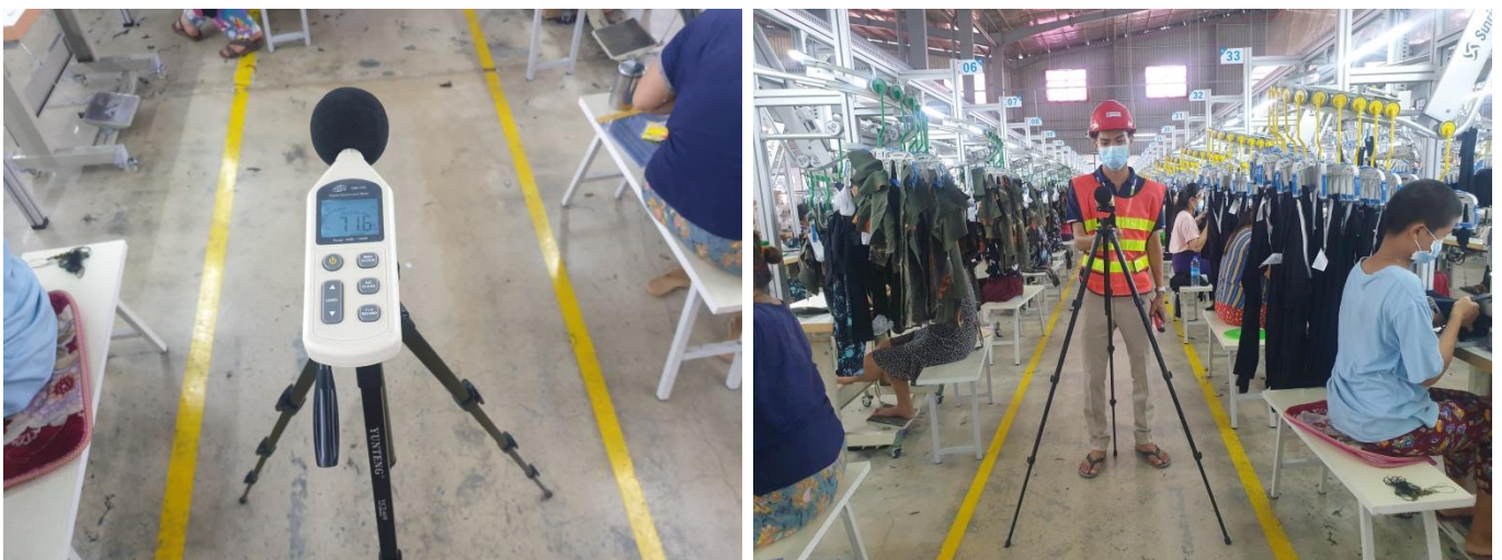
Figure 4-6 Sound level measurement photo
